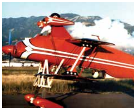
Craig Hosking's Doubletake incorporated landing gear on the top wing.
